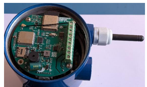
Figure 6: Attach the Antenna to the Device
