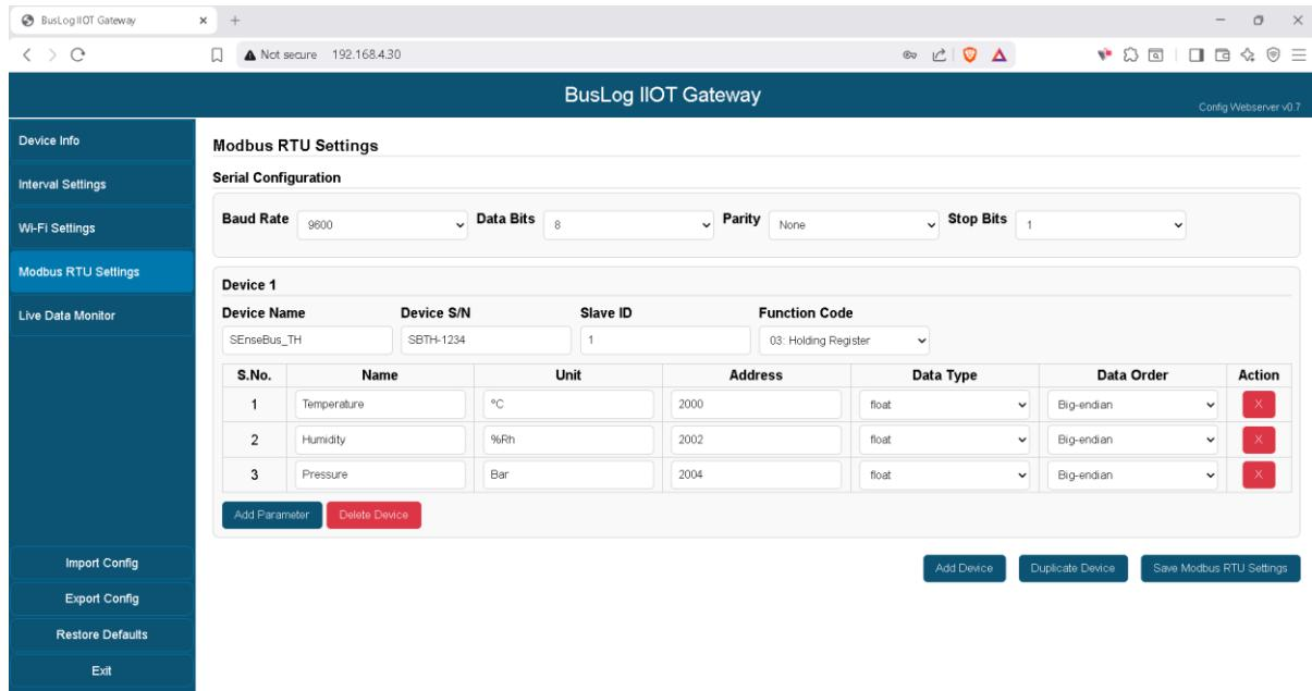
Live Data Monitor: Select the device to monitor and click the “Start Monitoring” button to read live Modbus parameters from the device to check the communication
