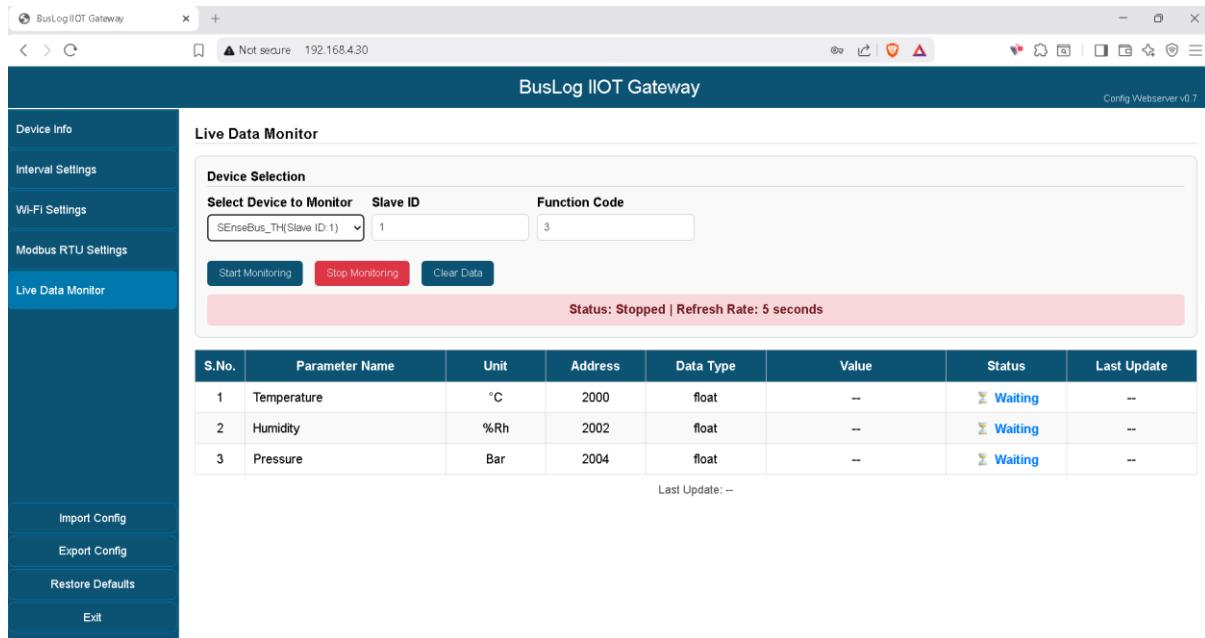
The screenshot shows the 'Live Data Monitor' section of the BusLog IIOT Gateway. The 'Device Selection' panel shows 'SEnseBus\_TH(Slave ID: 1)' selected with Slave ID 1 and Function Code 3. The 'Start Monitoring' button is highlighted in blue. The status bar at the bottom says 'Status: Stopped | Refresh Rate: 5 seconds'. The data table below shows three parameters: Temperature, Humidity, and Pressure, all in 'Waiting' status.
